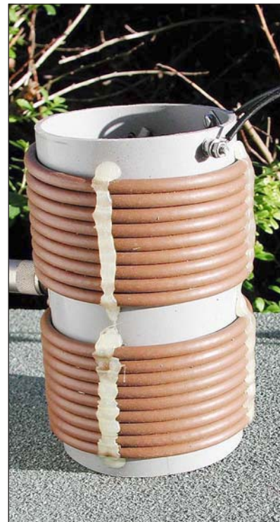
Top: A 7MHz loop using the 'comudipole' feed arrangement. The coax cable from the balun is connected to the coax output socket of the ATU.
